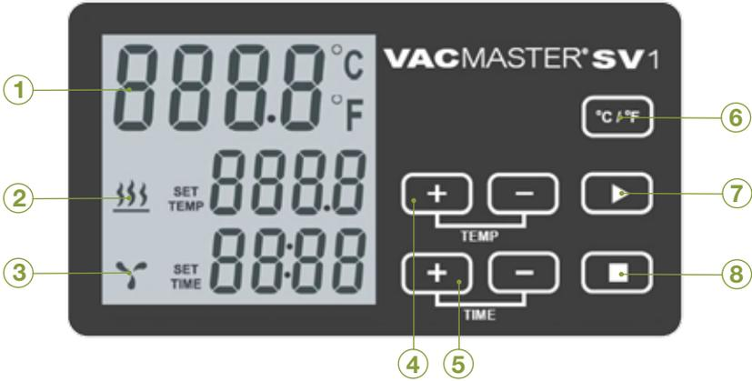
1. Water Temperature Display - Indicates the current water temperature.
