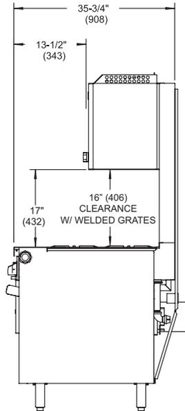
The broiler and flue riser assembly is shown here mounted on a six-burner open top range with a convection oven base.
